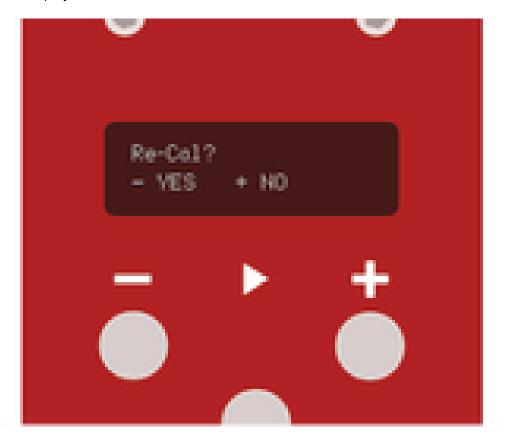
Press the *plus* button now to exit the recalibration program and restart the unit.
