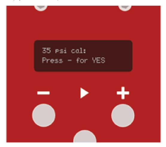
Attach your pump's nozzle to your reference tyre which has been inflated accurately to 35 psi. Press the *minus* button to proceed. This will recalibrate your Fumpa OG's internal digital gauge to the 35 psi value of the tyre.
