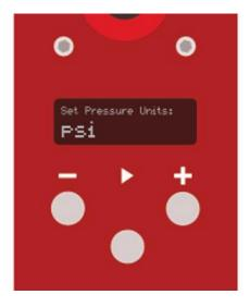
**Note:** Pressure unit selection is stored in Fumpa's memory. So, for example, if you select Bar as your pressure unit and turn Fumpa off, when you turn it back on again you will find Bar is still your default pressure unit.
