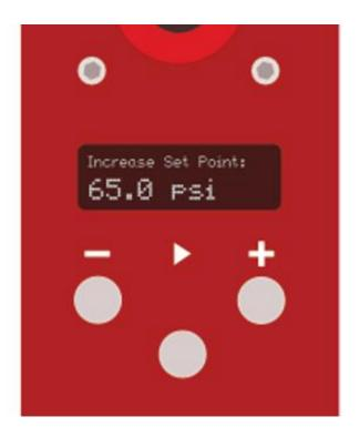
To use your Fumpa in manual mode just press and hold the 'play' button; Fumpa will start pumping and the OLED screen will display the current pressure. Releasing the 'play' button will stop Fumpa from pumping as you reach your desired inflation pressure.
