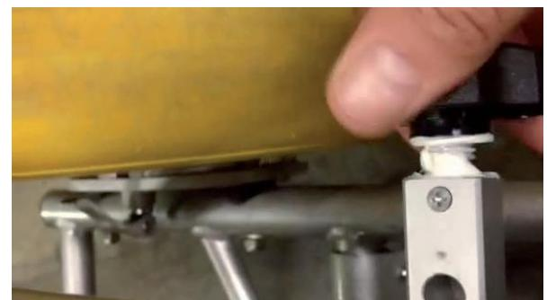
Loosen up the safety screw located on the housing of the floating arm chair
