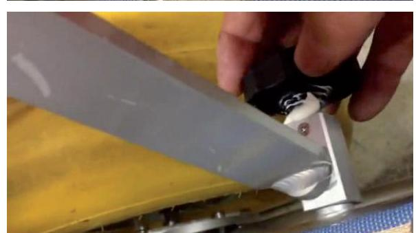
Pull down the chain that control the inclination of the back seat
